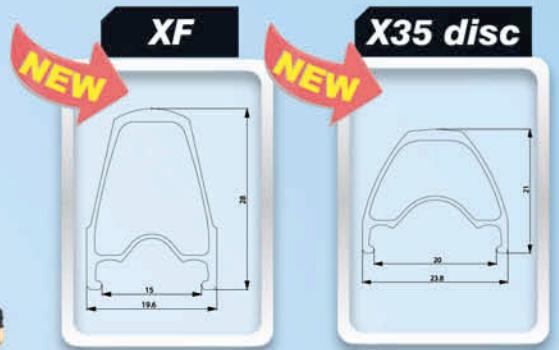
XF Alloy high 28mm Joint : weld 700C , 622X15 , 430g
