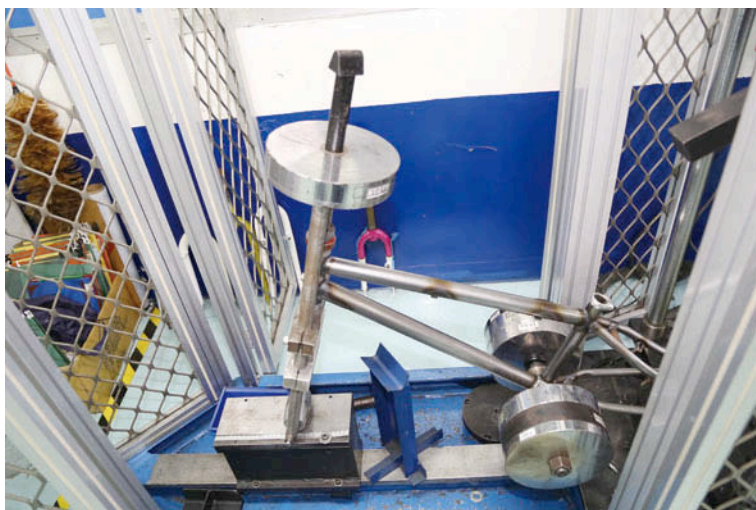
▲ La Bicycle puts its frames through rigorous testing.
