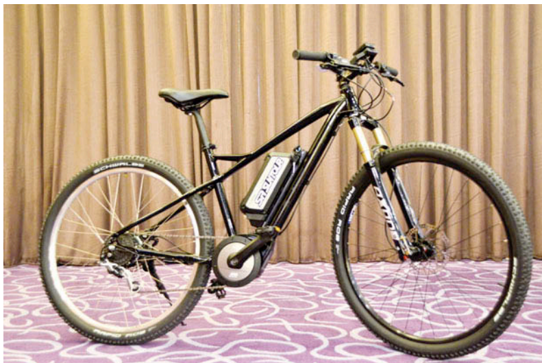
◀ SR Suntour's pedelec components can be used on 700C pedelecs (left) or e-MTBs (right), and the company's motors can drive either the front or the rear wheel.
