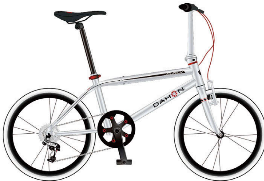
▲Dahon's Clinch uses an inverted handle post design to save weight.
