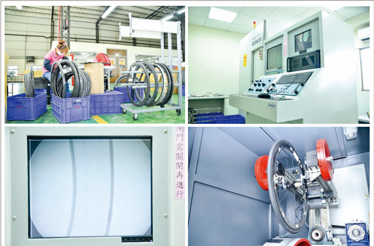
▲ ADK has its own rim factory. The factory's production processes are exacting, and x-ray machines are used to inspect products.
