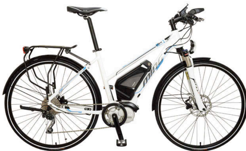
▲ Ming Cycle's 700C Pedelec uses Panasonic's 36V li-ion e-bike system.
