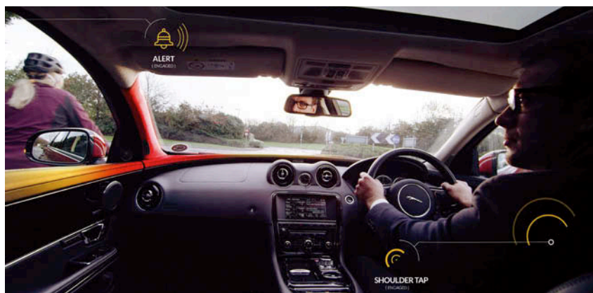
▲Jaguar's bike Sense detects when cyclists approach and warn the driver with a matrix of amber and red led lights.
