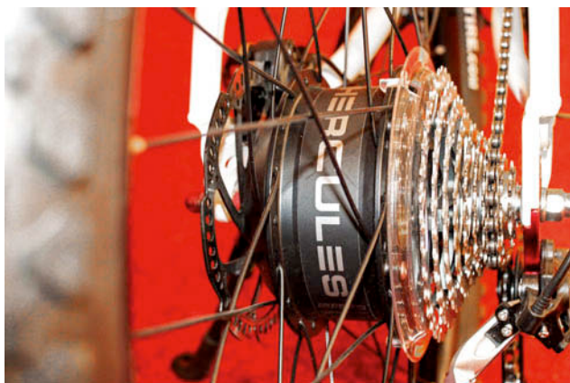
▲ For E-MTBs, SR Suntour's rear wheel drive motor offers outstanding heat dissipation properties.
