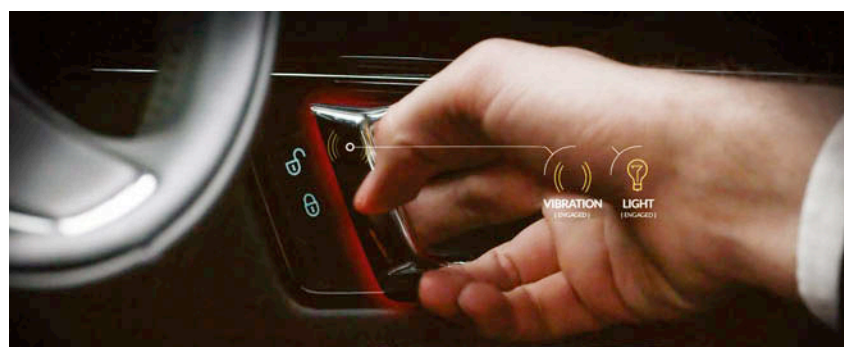
▲Door handles will light up and vibrate if the driver tries to open a door when Bike Sense detects a passing cyclist.
