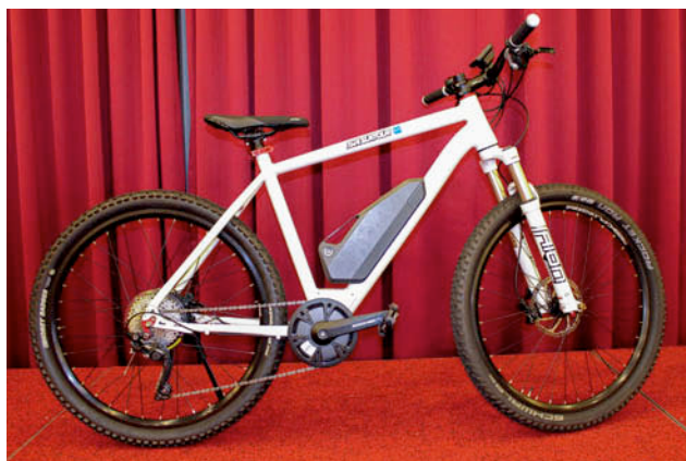
▲ With the sensor integrated into the large chainring, and the control box integrated into the battery the whole bike has a sleek and tidy appearance.
