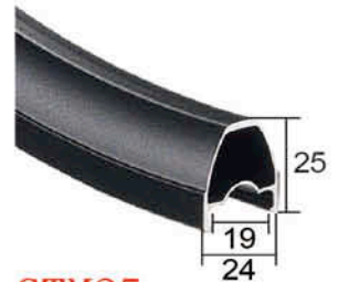
GTM25 Joint:Sleeved 29",622x19-490g 27.5",584x19-470g
