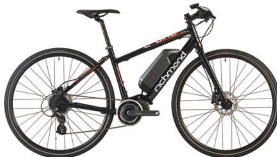
◀ E-STRADA 6.0 TREKKING w/Shimano E-6000 Steps With 250W/36V Electric Drive Unit 418Wh capacity lithium-ion battery
