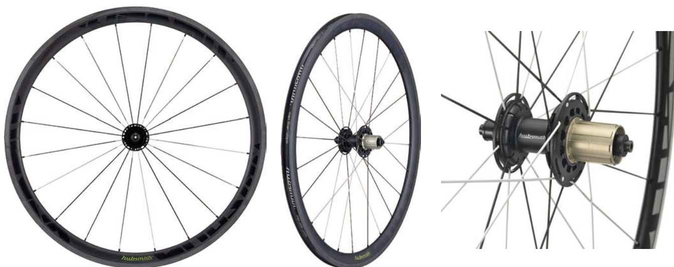
▲HS-Titan CC38 wheels employ a patented double-layer weave construction, and are paired with patented double-layer weave hubs.
