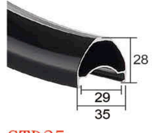
GTD35 Joint:Weld / Sleeved 29",622x29-535g 27.5",584x29-520g
