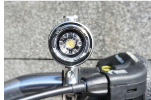
▲ The dual function safety device is both bell and light.
