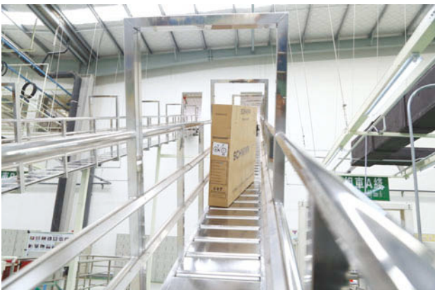
▲ Bicycle boxes are sent down a conveyor from an upper floor saving workshop space, time and man hours.
