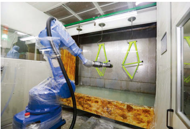
▲ Automated mechanical arm on painting line.
