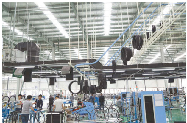
▲ Rims are transported along an elevated conveyor line.
