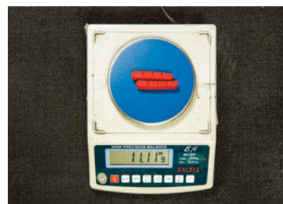
▲ Measurement of brake shoe weight before and after testing enabled the brake shoe wear rate to be determined. (Image is a photograph taken at this laboratory.)
