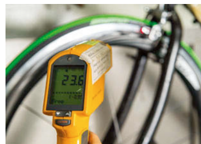
▲ A non-contact infrared temperature measure system was used to record the highest temperature during the testing process.
