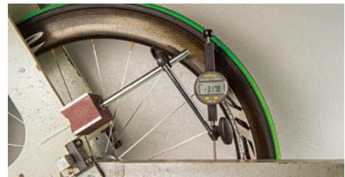
▲ Measurement of the displacement of the jig and rim enabled the rigidity of the rear wheel during cycling to be determined.
