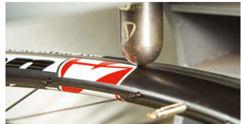
▲After a 20 kg force was applied to the rim, rim deformation was measured; the greater the resulting value, the better the rigidity.
