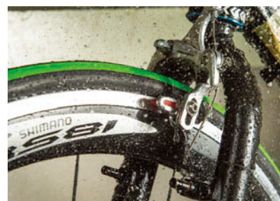
▲ Water was sprinkled to simulate riding on a rainy day when measuring wet braking force.
