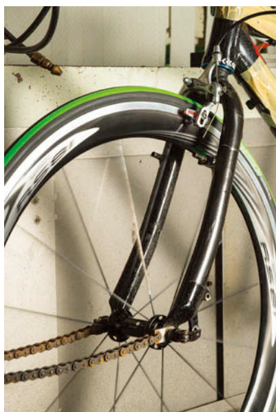
▲ Dry braking force was measured to obtain the braking force of the wheels and brake shoes.
