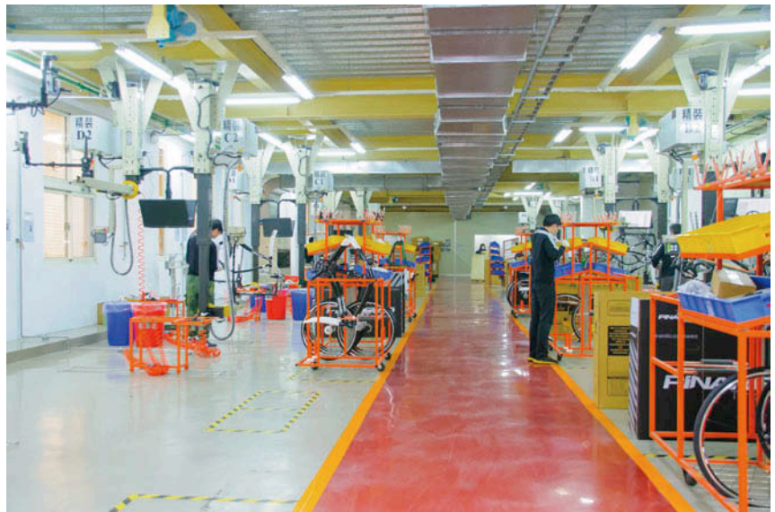
▲ The adoption of RFID management of production processes and a work station assembly format allows Fritz Jou to fill both large and small orders with flexibility and efficiency.
