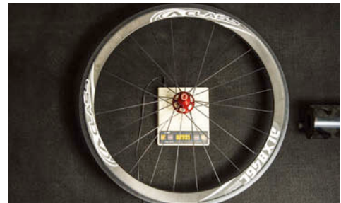
▲ Measurement of the displacement of the jig and rim enabled the rigidity of the rear wheel during cycling to be determined.
