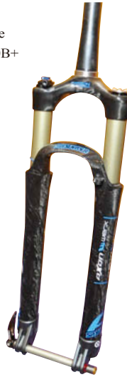
◀The steerer tube, crown and legs of Axon Werx F have been upgraded to carbon fiber material. The 27.5-inch version now weighs 1,482 grams.
