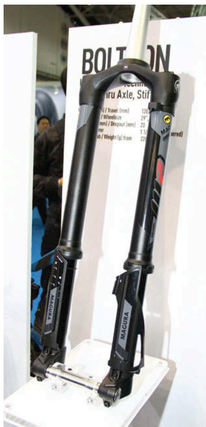
▲Magura Boltron eMTB specific upside down fork.
