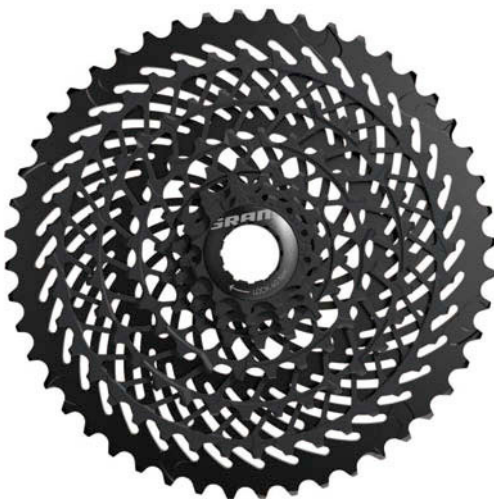
▲SRAM's 8-speed (11-48T) E-Block cassette.
