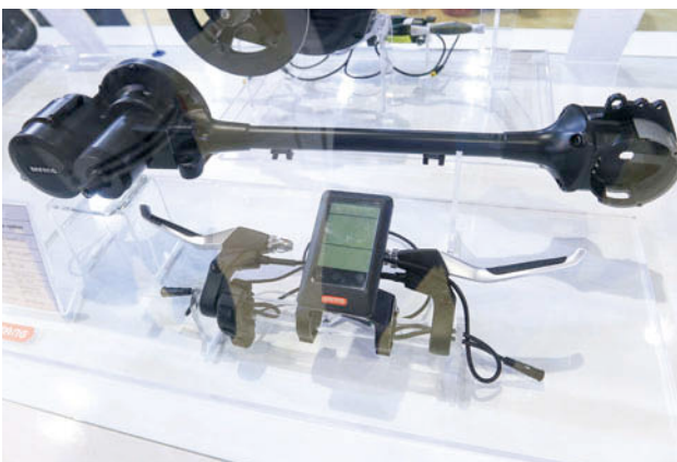
▲ Bafang's shaft drive shift showcased a possible future direction for e-bikes.
