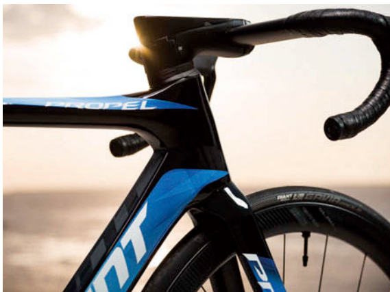
▲Propel Advanced SL Disc bar and stem: The new Propel Advanced SL Disc model shown here features a Giant Contact SLR Aero handlebar-and-stem unit with internal cable routing. Cameron Baird photo.
