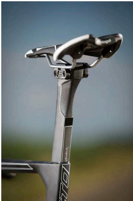
▲ The new S-Flex seatpost offers a slimmer cross-section.
