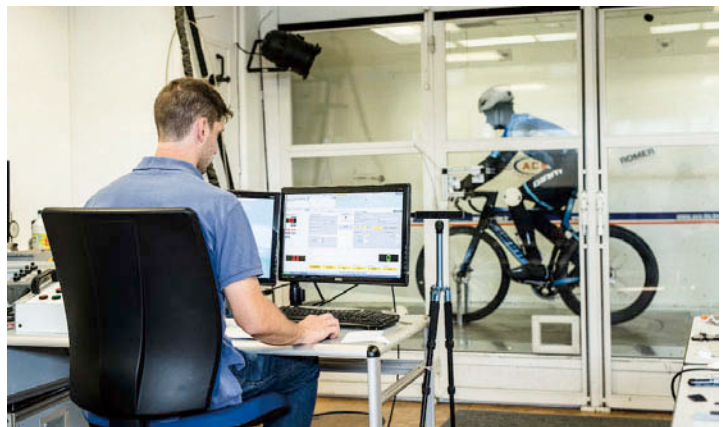
▲Propel Disc ACE Wind Tunnel: To ensure the most efficient aerodynamic design and performance, Giant engineers built their own mannequin—the first in the bike industry to do so. The Aero Concept Engineering facility in Magny-Cours, France served as the site for final tests and development.
