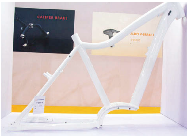
▲ Guangzhou Leonis' mid motor frame, can be equipped with a belt drive system.
