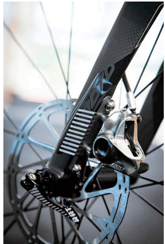
▲ Disc-brake models include Merida's disc cooler heat sinks.
