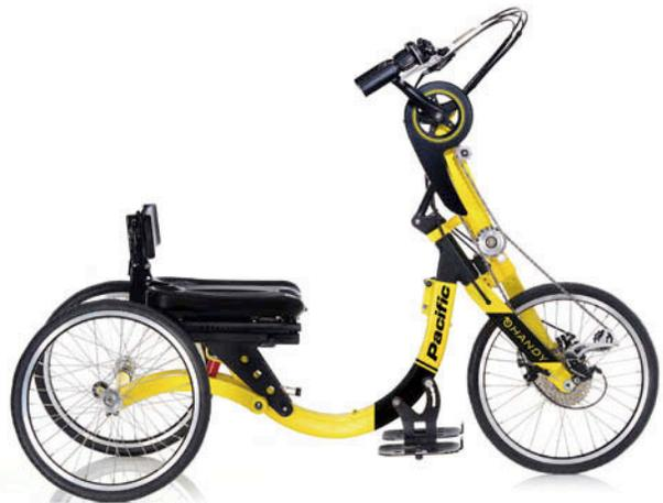
1/6 of leg power output. This handcycle motor system provides an optimized assisting power while cycling with both hands simultaneously. Finally, elastomer suspension is designed onto the frame to bring comfort, stability, and a big smile on users' face!
