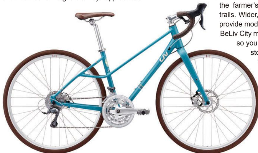
Dual-position brake levers allow for easy access to powerful disc brakes. So, you can stop safely from the tops of the bars, the hoods or the drops — rain or shine.
