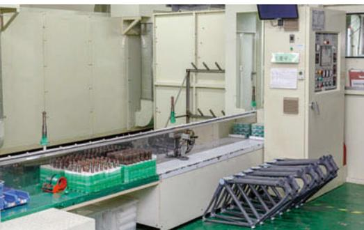
▲ Automatic electrostatic coating system helps to reduce the inconsistencies found in the manual process.
