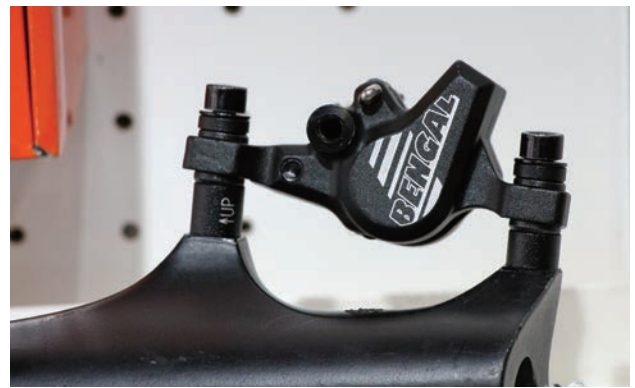
▲ With the addition of only a few small parts, Bengal's PM7 and PM8 adaptor base allows calipers for 180mm brake discs to accept 200mm or 203mm discs.
