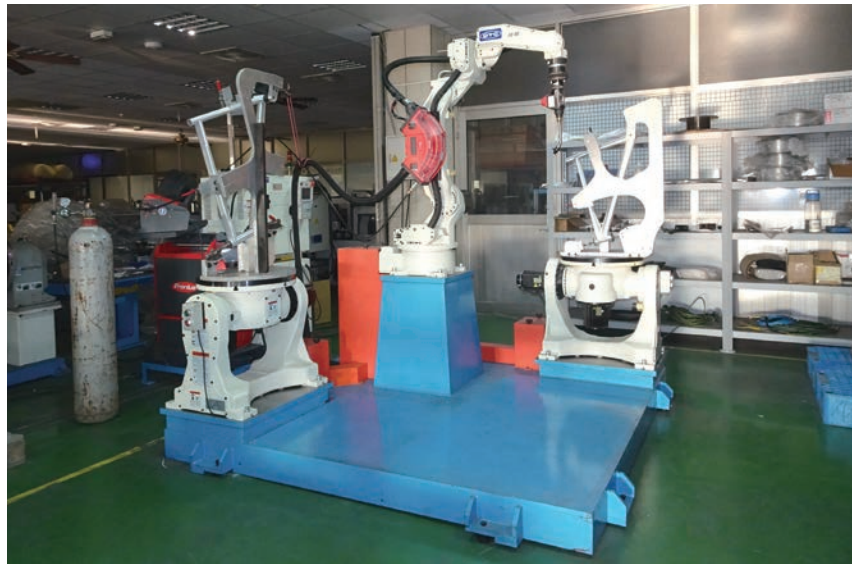
▲ Automatic MIG welding equipment. In today's era of high labor wages, the automatic and precise welding of robots will increase productivity and reduce labor costs for the frame factory, making the products more competitive.
