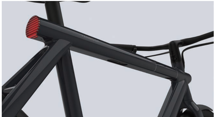
▲ The frame's 166 responsive LED's give information to both rider and other road users.
