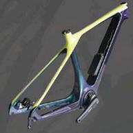
PEL210028 Carbon Frame For E-BLKi Size: 27.5' Seat post: 31.6mm Seat Clamp: 35mm
