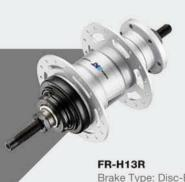
Brake Type: Disc-Brake O.L.D: 135mm Weight: 1050g
