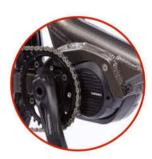
Motor housing compatible with Shimano DU-E8000.
