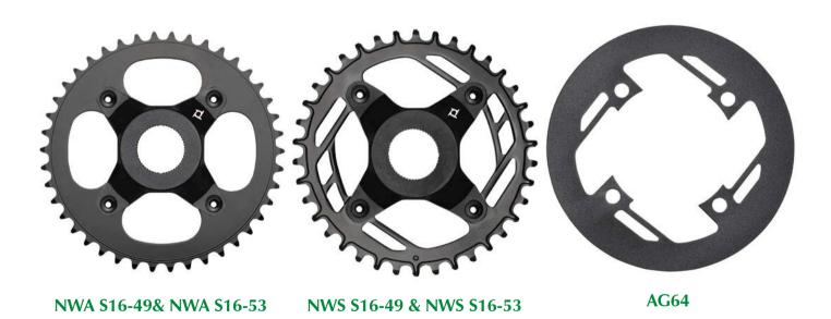
The chain wheel set is compatible with 11s, 12s. The narrow chaining design avoids chains dropping off and has an alloy chain guard option with various chaining choices. Chaining from  $32T \sim 40T$ , both steel and alloy 7075 have chainlines of 49mm and 53mm.
