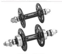
GT-002F Body Material: AL6061 Axie Material: CR-MO O.L.D: 100mm Spoke: 14g\*24/28/32/36H Weight: 236g Bearing: Sealed Bearings x2 GT-002R AL6061 CR-MO 120mm 14g\*24/28/32/36H
