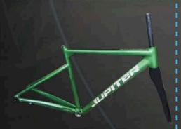
PEL210029 Alloy Frame+Carbon Fork Size: 700C Material: Alloy 6061
