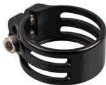
● Item No: HK-050G Material:AL6061T6 Full CNC Bolt:Cr-mo Dia: 34.9mm Length:20.0mm Finish:Silver OR ED Black
