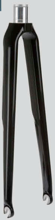
FK-34AC-QR ALLOY CARBON RACING / FIXIE / TRACK FORK STEM : ALLOY / 1-1/8 AXLE-TO-CROWN : 363MM -370MM BRAKE : CALIPER BRAKE / NO BRAKE HOLE DROP OUTS : 9MM * 100MM QR RAKE : 35MM -40MM
