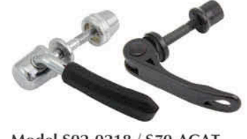
Model S02-0218 / S70-AGAT Type: Seat Pin Q,R Material: Axle is Cr-mo, Axle Diam: M6 or M8 / M6 Length(L):25, 28, 30, 35, 40, / 28, 33 Length(B):45, 48, 50, 55, 60, / 43, 48 Weight:94g/ 38g
