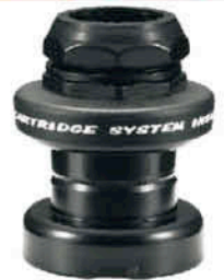
CH-9072BW 1", ROTATE 130 Ø 22.2x30x27
