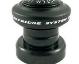
CH-9072TBW 1", ROTATE 130° Ø 25.4x30x27 Material : Alloy(#1.2), Rubber(#B), Steel(#3.4.5) Type : Threadless, Cartridge Height : 15+12.3=27.3mm Weight : 155g
