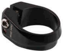
● Item No: HK-050F Material:AL6061T6 Full CNC Bolt:Cr-mo Dia:31.8 / 34.9 / 36.0mm Length:21.0mm Finish:Silver OR ED Black
