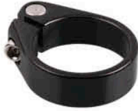
● Item No: HK-050B Material:AL6061T6 Bolt:Cr-mo Dia:28.6 / 31.8 / 34.9mm Length:13.0mm Finish:Silver OR ED Black
