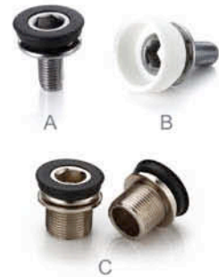
Model : SHL 08 Cotterless axle bolt for chain wheel Size : A、B : M8*1.0*15~22mm C : M15*1.0*13.5mm Material : SCM435 SUS304
