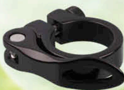
● Item No: HK-051F Material:AL6061T6 Lever NC Bolt:Cr-mo Dia:28.6 / 31.8 / 34.9mm Length:13.0mm Finish:Silver OR ED Black
