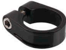
● Item No: HK-050C Material:AL6061T6Forged Bolt:Cr-mo Dia:28.6 / 31.8 / 34.9mm Length:15.0mm Finish:Silver OR ED Black
