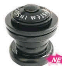
CH-664TBW 1" Ø 25.4x30x27 Material : Alloy(#1), Nylon(#A-1,5-1), Steel(#A.2.3.4.5) Type : Threadless, Ball Retainer Height : 14.5+10.5=25mm Weight : 135g
