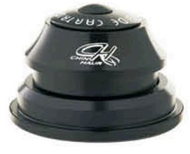
CH-6255TEBW UPPER 1-1/8", LOWER 1-1/2" Ø 28.6x44x55x39.8 Material : Alloy(#1), Nylon(#2,B), Steel(#3.4.5) Type : Threadless, Cartridge Height : 15+4=19mm Weight : 155g CH-6256TEBW -> #5: Ø30.0mm
