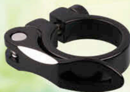
● Item No: HK-051G Material:AL6061T6 Bolt:Cr-mo Dia:28.6 / 31.8 / 34.9mm Length:13.0mm Finish:Silver OR ED Black
