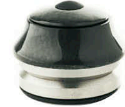
CH-990TEBW CARBON, 1-1/8" Ø 28.6x41.8x30 Material : Carbon(#1.2), Nylon(#B), Steel(#5) Type : Threadless, Sealed Bearing Height : 10.5+0.8=11.3mm CH-990TBW #2-> 8.6mm CH-990TEBW #2-> 15.8mm CH-990TBW #2-> 25.8mm
