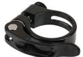
● Item No: HK-051I Material:AL6061T6 Bolt:Cr-mo Dia:28.6 / 31.8 / 34.9mm Length:13.0mm Finish:Silver OR ED Black
