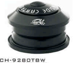
CH-9280TBW 1-1/8" Ø 28.6x44x30 Material : Alloy(#1), Nylon(#2,B), Steel(#3.4.5) Type : Threadless, Cartridge Height : 9.2+3=12.2mm Weight : 133g CH-9280TEBW #2-> 15mm CH-9280TBW #2-> 20mm CH-9280TBW #2-> 30mm
