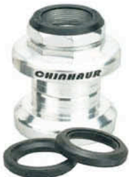
CH-105AW 1" Ø 22.2x30x27/30.2x26.4 Height : 25+12.2=37.2mm Weight : 110g
