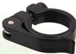
● Item No: HK-051A Material:AL6061T6 Bolt:Cr-mo Dia:28.6 / 31.8 / 34.9mm Length:13.0mm Finish:Silver OR ED Black
