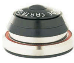
CH-6502TBW UPPER 1-1/8", LOWER 1-1/2" Ø 28.6x41.8x52x39.8 Material : Alloy(#1.2), Nylon(#B), Steel(#5) Type : Threadless, Sealed Bearing Height : 10.5+0.8=11.3mm Weight : 110g CH-6502-1TBW -> #5: Ø30.0mm
