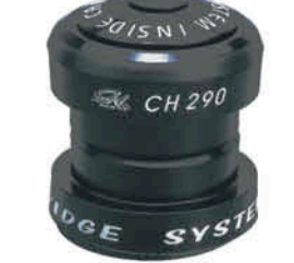
CH-290TBW 1-1/8" Ø 28.6x34x30 Material : Alloy(#1.2), Nylon(#B), Steel(#3.4.5) Type : Threadless, Cartridge Height : 13+10=23mm Weight : 132g
