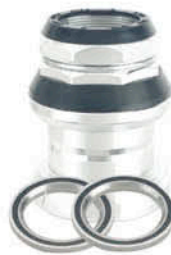
CH-106AW 1" Ø 22.2x30x27/30.2x26.4 Height : 27.5+10.8=38.3mm Weight : 85g
