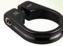
● Item No: HK-050D Material:AL6061T6NC Bolt:Cr-mo Dia: 31.8 / 34.9mm Length:11.0mm Finish:Silver OR ED Black
