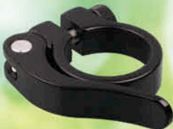
● Item No: HK-051E Material:AL6061T6Lever NC Bolt:Cr-mo Dia:28.6 / 31.8 / 34.9mm Length:13.0mm Finish:Silver OR ED Black
