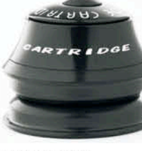
CH-918TEBW 1-1/8" Ø 28.6x44x30 Material : Alloy(#1.2), Nylon(#B), Steel(#3.4.5) Type : Threadless, Cartridge Height : 17.5+3=20.5mm Weight : 148g
