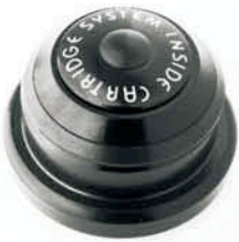
CH-600TBW UPPER 1-1/8", LOWER 1-1/2" Ø 28.6x44x49.7x39.8 Material : Alloy(#1.2), Nylon(#B), Steel(#3.4.5) Type : Threadless, Cartridge Height : 9.2+11.2=20.4mm Weight : 206g
