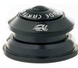
CH-6201TBW UPPER 1-1/8", LOWER 1-1/2" Ø 28.6x44x56x39.8 Material : Alloy(#1.2), Nylon(#B), Steel(#3.4.5) Type : Threadless, Cartridge Height : 9.2+4=13.2mm Weight : 165g CH-6201-1TBW -> #5: Ø30.0mm
