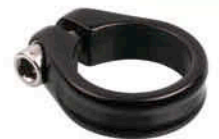
● Item No: HK-050J Material:AL6061T6 Forged Bolt:Cr-mo Dia: 28.6 / 31.8mm Length:13.0mm Finish:Silver OR ED Black
