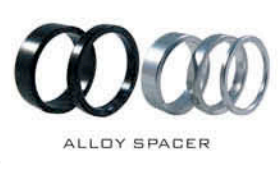
CH-290TBW 1-1/8" Ø 28.6x34x30 Material : Alloy(#1.2), Nylon(#B), Steel(#3.4.5) Type : Threadless, Cartridge Height : 13+10=23mm Weight : 132g
