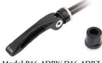
Model B16-ADBY/ D16-ADBZ Type: Hub Q,R Material: Axle is AL7075 Axle Diam: B:9mm, D:10mm Length(L): B=112,D=148.5 Weight:64g/ 79g
