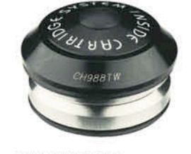
CH-988TBW 1-1/8" Ø 28.6x41.8x30 Material : Alloy(#1.2), Nylon(#B), Steel(#5) Type : Threadless, Sealed Bearing CH-988TBW #2-> 8.6mm CH-988TEBW #2-> 15.8mm CH-988TBW #2-> 25.8mm
