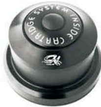
CH-6381TBW UPPER 1-1/8", LOWER 1-1/2" Ø 28.6x44x49.7x39.8 Material : Alloy(#1), Nylon(#2,B), Steel(#3.4.5) Type : Threadless, Cartridge Height : 9+11.2=20.4mm Weight : 199g CH-6382TBW -> #5: Ø30.0mm
