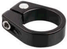
● Item No: HK-050A Material:AL6061T6 Bolt:Cr-mo Dia:28.6 / 31.8 / 34.9mm Length:13.0mm Finish:Silver OR ED Black
