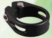
● Item No: HK-050E Material:AL6061T6Full CNC Bolt:Cr-mo Dia:31.8 / 34.9 / 36.0mm Length:14.0mm Finish:Silver OR ED Black
