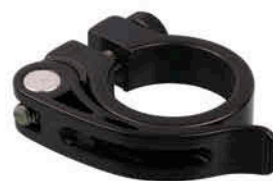
● Item No: HK-051C Material:AL6061T6 Bolt:Cr-mo Dia:28.6 / 31.8 / 34.9mm Length:13.0mm Finish:Silver OR ED Black
