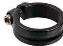
● Item No: HK-050I Material:AL6061T6 Forged Bolt:Cr-mo Dia: 34.9mm Length:14.0mm Finish:Silver OR ED Black
