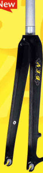
▲ FRC-621 1-1/8" alloy steerer, N47 crown, PM disc brake
