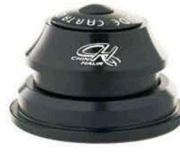
CH-6202TEBW UPPER 1-1/8", LOWER 1-1/2" Ø 28.6x44x56x39.8 Material : Alloy(#1.2), Nylon(#B), Steel(#3.4.5) Type : Threadless, Sealed Bearing Height : 15+4=19mm Weight : 145g CH-6202-1TEBW -> #5: Ø30.0mm
