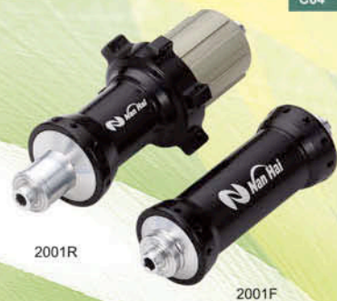
NH-2001R /2001F (4 Sealed) Spoke Hole: ( F ) 18/20/24H, ( R ) 24H Axle Dim: ( F ) \Phi 9x100x110mm ( R ) \Phi 10x130x140mm Flange PCD: ( F ) 35mm, ( R ) 39-50,57mm Weight: ( F ) 103g, ( R ) 221g
