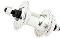
FD-130 (Disk) For MTB-Disk, Nut Type Alloy Body, 28H / 32H / 36H. Flange Space : 58mm Flange PCD : 58mm
