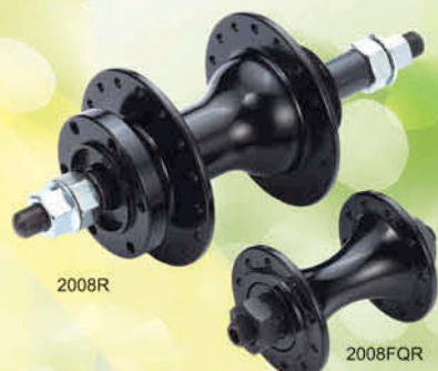
NH-2008R /2008FQR (LOOSE BALL) Spoke Hole : 20/28/32/36H O.L.D.: (F) 72,75mm/ (R) 135mm Axle Length: (F) 110/115/120/125mm (R) 145mm
