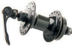
FD-130QR (Disk) For MTB-Disk, QR Type Alloy Body, 28H / 32H / 36H. Flange Space : 58mm Flange PCD : 58mm
