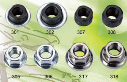
NH-301/302/307/308/305/306/317/318 301: Front hub cone 5/16" 302: Rear hub cone 3/8" 307: Front hub cone QR M9 308: Rear hub cone QR M10 305: Front nut and washer 5/16 X26T 306: Rear nut and washer 3/8 X26T 317/318: Anti-scratching heavy load nut, M9/M10, 3/8"26T
