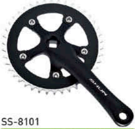
SS-8101 Steel or alloy chainwheel with alloy crank. Chainring: 36, 38, 39, 42, 44T Crank: Alloy 165, 170, 175mm (5-arm) BCD: 110mm Chainline: 43mm Axle length: 103mm
