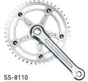
SS-8110 Chainring: 44, 46, 48, 50, 52T. Alloy Crank: Forged 6066/T6 alloy Length: 165, 170mm BCD: 144mm Axle length: 103mm
