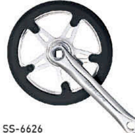
SS-6626 Steel chainwheel & double chaincover with cotterless crank. Chainring: 36, 38, 40, 44T Crank: 5", 5-1/2", 6", 170mm Chainline: 45mm Axle length: 119mm
