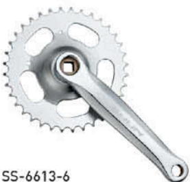
SS-6613-6 Steel chainwheel with steel cotterless crank. Chainring: 28, 30, 32, 36, 38T Crank: 152, 165, 170mm Chainline: 45mm Axle length: 127.5mm
