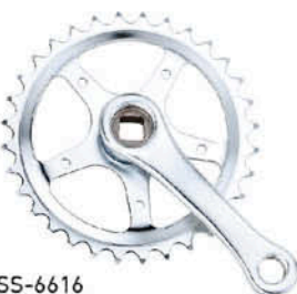
SS-6616 Steel chainwheel with steel cotterless crank. Chainring: 26, 28, 32, 33T Crank: 4", 5", 5-1/2" Chainline: 45mm Axle length: 120mm
