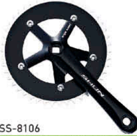
SS-8106 Chainring: 39, 42, 44, 46, 48, 50, 52T. Steel or alloy Crank: Forged 6061/T6 alloy Length: 165, 170, 175mm BCD: 130mm Chainline: 43mm Axle length: 103mm
