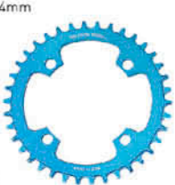
MTB-03 Narrow wide tooth. For 9-12s BCD: 104mm. Chaining: 30, 32, 34, 36, 38, 40, 42T Chainline: 50.5mm. (48.5mm for 30T)
